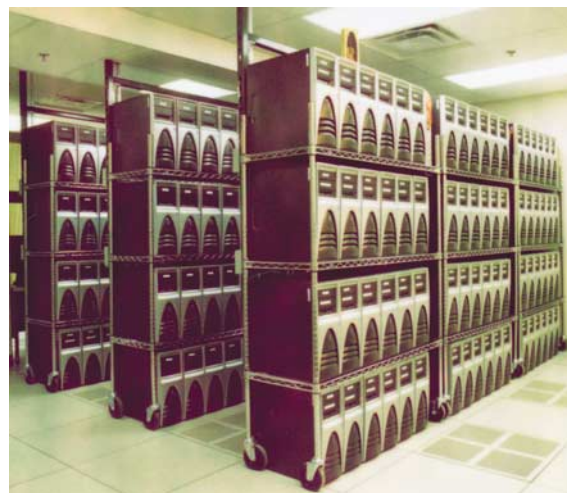
Figure 1 Kibbutz100, a homemade 1.1 teraflops supercomputer for virtual screening and multiple molecular dynamics simulations.
