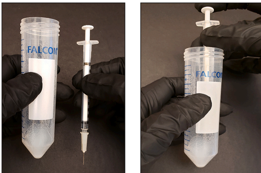
Figure 3. Ensuring minimal buffer carry over to the next step during resin preparation
