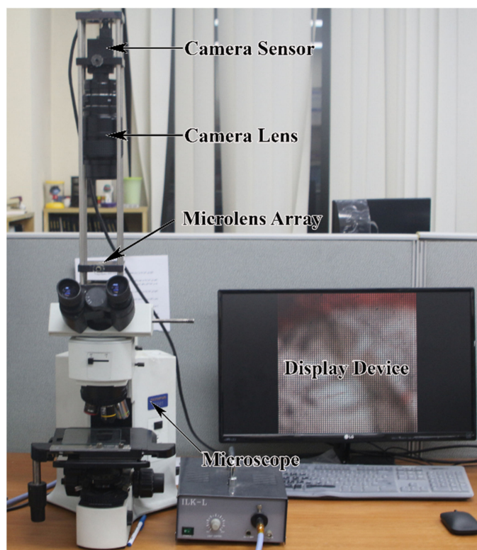
Figure 6. Experimental setup for the proposed IIM resolution enhancement system. The microlens array (MLA) is placed between the camera sensor and the specimen, and the captured EIA is displayed in the display in real-time.
