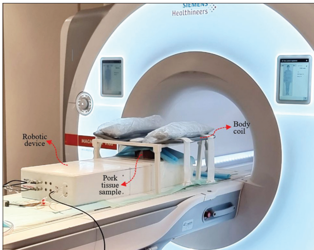
Figure 2: Experimental setup for grid ablation in tissue-mimicking phantom/porcine tissue sample arranged on the table of a 3T magnetic resonance imaging scanner, with the key components indicated
