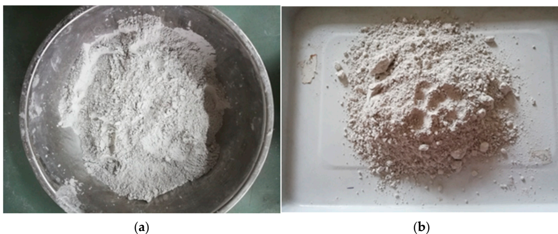
Figure 15. Raw materials. (a) UCCG (b) GGBFS powder.
