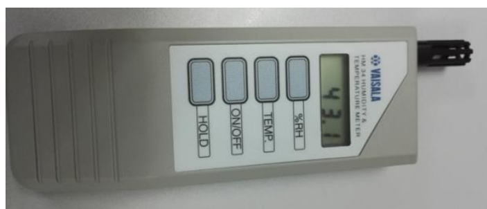
Figure 3. Standard temperature and humidity sensor.
