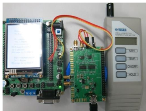
Figure 13. Prototype sensor with LCD display module (Left), PCB integration of sensor device and ASIC (Middle) and standard humidity sensor (Right).
