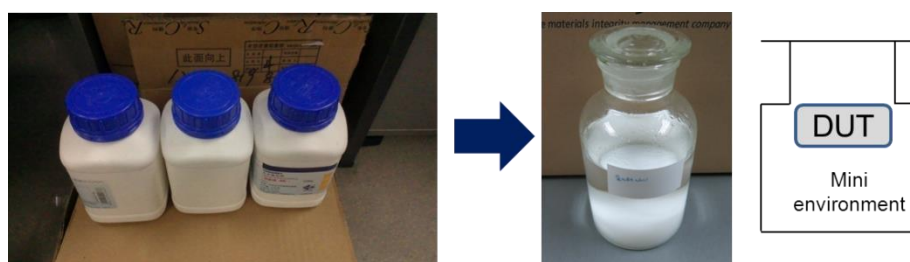
Figure 4. Mini-environment built with a saturated salt solution sealed in glass chamber.
