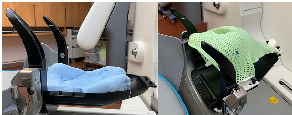
FIGURE 1: Mask adapter for GK Icon. The water-activated polystyrene cushion (left) is custom shaped to a suitable head positioning for the patient. The cushion rests within the mask adapter, which has an indexing indentation visible in the right image to hinder cushion translation along the craniocaudal (z) axis. White lines on the adapter define the optimal treatment space for head positioning. A three-point aquaplast mask (right) is used for head immobilization. A submental mask lip helps prevent uncomfortable mask fitting. A nose opening is formed, allowing placement of an optical marker.
