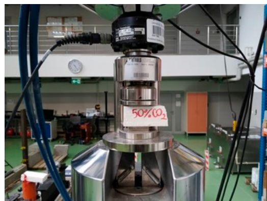
Figure 3. Compressive strength test conducted on the 50% CO 2 sample after 28 days.
