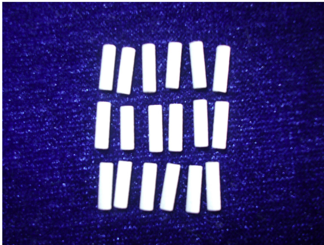
Fig. 1. The coatings/Ti-6Al-4V substrate composition cylindrical samples used in experiments in vivo .
