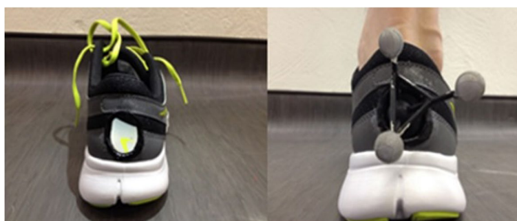
Fig. 3 Customised neutral shoes (Nike® model Flex Experience RN 2 MSL ) with opening in posterior region to allow cluster to be attached directly to calcaneus for kinematic analysis
