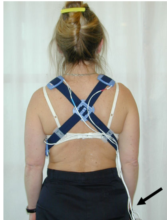
Fig. 2 The harness with embedded electrodes for EMG recording of the upper trapezius. The EMG logger and feedback device was carried in a small pouch (see arrow)
