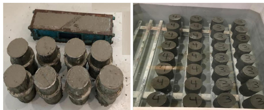
Figure 1. Concrete cylinder and beam specimens.
