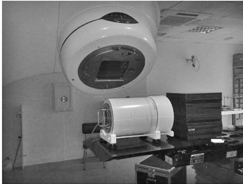
FIG. 1. Picture of the experimental setup. This setup includes a stand made of carbon fiber in order to avoid the influence of the treatment couch and a microchamber placed inside an acrylic insert for isocenter dose measurement.
