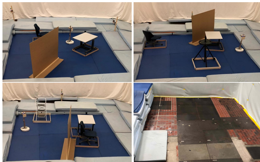
Figure 5. Three out of ten setups for data collection using the modified spline antenna are shown. In each setup the Roomba robot drove a different trajectory and the obstacles' or the transmitters' location was changed. The picture in the bottom right shows the floor made of ceramic tiles and metal plates.
