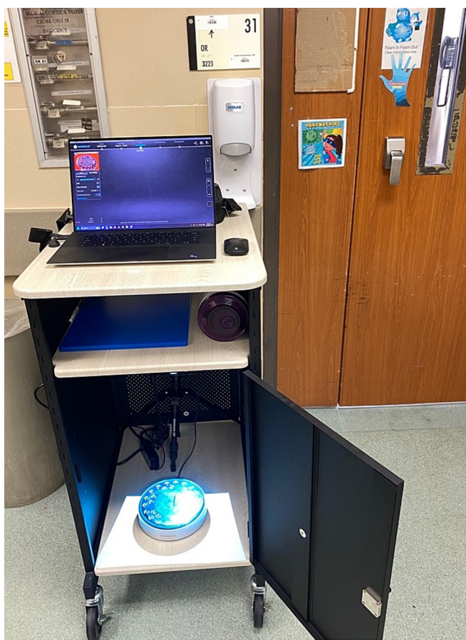
Fig. 1. Mobile 3D scanning cart that may be set up outside of the OR (shown here) or pathology lab. Scanning occurs in the lower compartment of the cart and the door is closed to ensure optimal dark conditions for 3D scanning.
