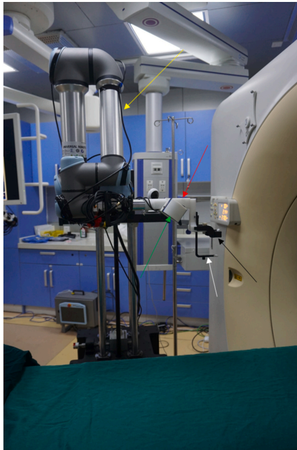
Fig. 3. Connection between the mechanical arm and the needle holder: mechanical arm (yellow arrow), clamping arm of the radiopaque needle holder (red arrow), rear needle holder (black arrow) for entering the needle, front needle holder (white arrow) for avoiding the bending of the puncture needle, and one of the laser beam modules (green arrow). (For interpretation of the references to colour in this figure legend, the reader is referred to the Web version of this article.)
