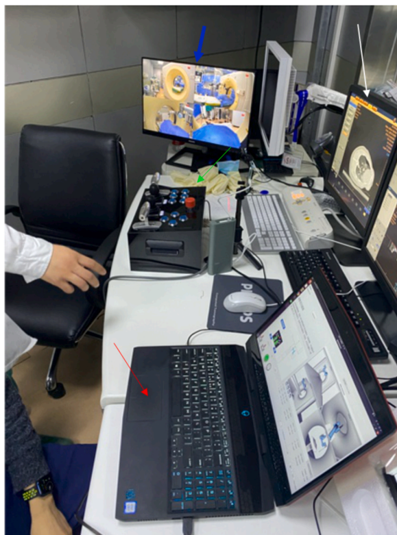
Fig. 2. Layout of the remote control compartment: remote-controlled console (green arrow), the red button on the console is the emergency stop button; monitor of CT (white arrow), robot monitoring system (blue arrow), and control host of the robot (red arrow). (For interpretation of the references to colour in this figure legend, the reader is referred to the Web version of this article.)
