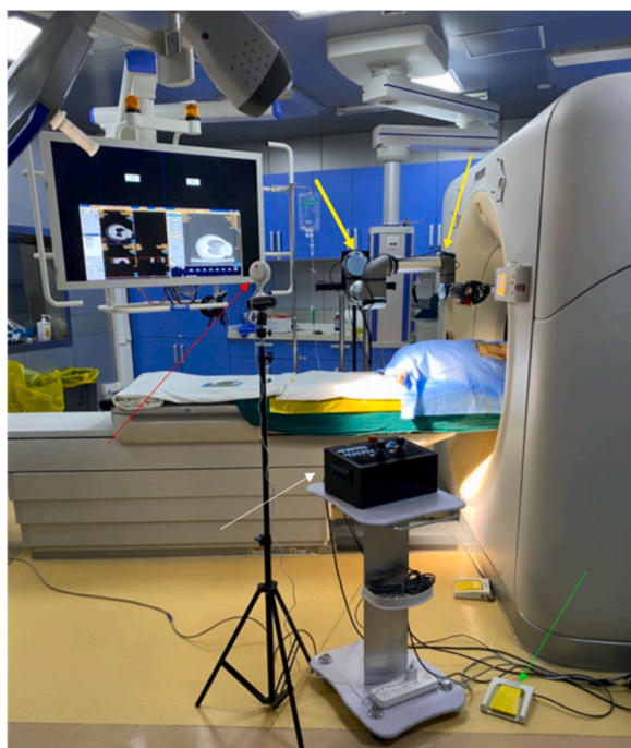
Fig. 1. Layout of the robot near the CT bed: robot manipulator (yellow arrow), movable remote control console (white arrow), monitoring camera of the robot system (red arrow), and pedal (green arrow). (For interpretation of the references to colour in this figure legend, the reader is referred to the Web version of this article.)
