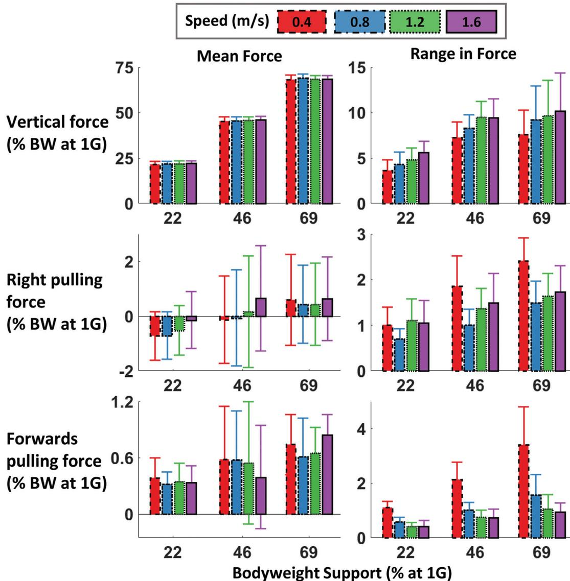
Fig. 4 Mean and range (with standard deviations) of support force over a stride at four speeds
