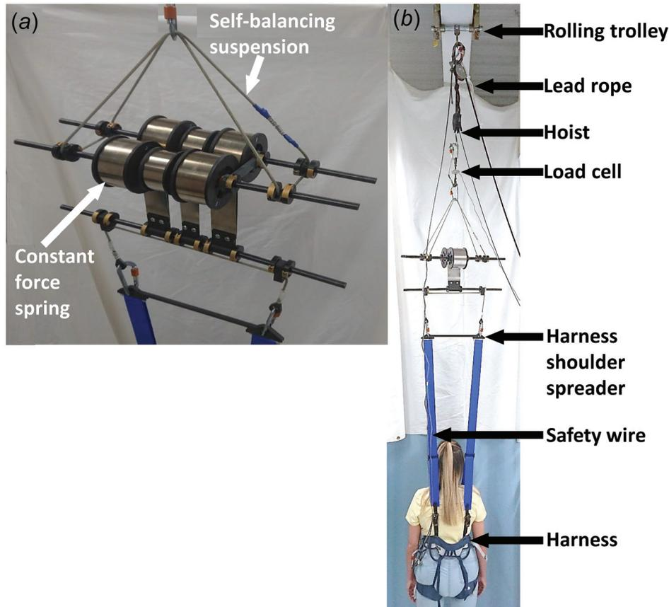
**Fig. 1 The bodyweight support system we designed. Image (a) shows the main section of the system with three pairs of constant force springs. The entire support system, with just one spring pair, is shown in image (b).**
