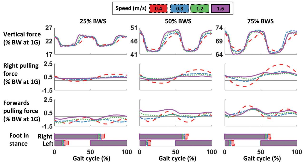
Fig. 3 Vector decomposition of the support force from the bodyweight support system over a stride at four speeds as found by loadcell measurements and kinematic positions
