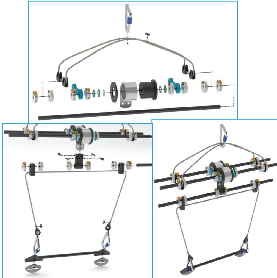
**Fig. 2** Breakdown on the components used to build the main part of a single spring pair system. Top is the components that are slid and locked into place on each of the two top bars. Bottom left is how we assembled the bottom section of the system. Bottom right is the fully assembled spring system.
