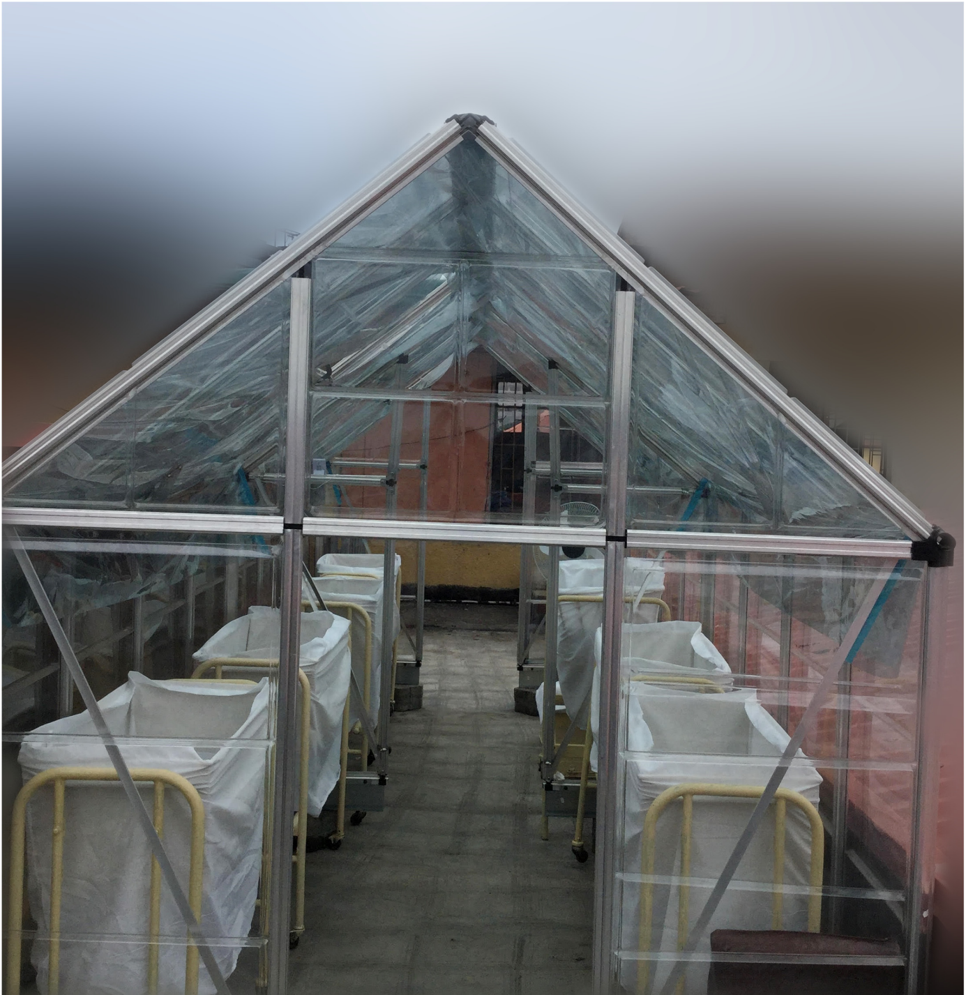
Fig 1. Proposed filtered sunlight phototherapy enclosure with embedded films.
