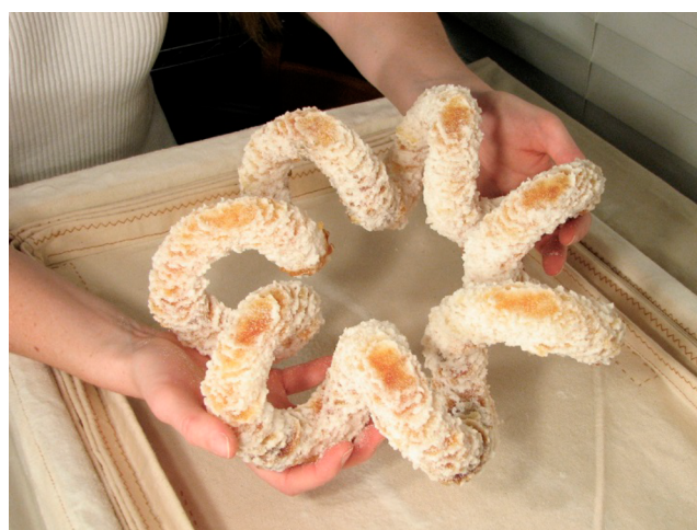
Figure 70. Sugar sculpture produced by means of SLS (CandyFab Sugar Printing; image by Windell H. Oskay). 721 License CC BY 2.0.
