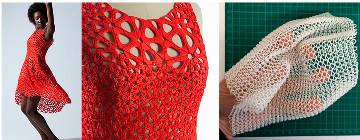
Figure 78. Flexible textiles by AM. Left and center: The Kinematics Dress 6 from Nervous System (dress designed by Jessica Rosenkrantz and Jesse Louis-Rosenberg; photos by Steve Marsel Studio; images reproduced with permission from Nervous System). 799 Right: Weft knitted PA-12 textile produced by SLS. 803 License CC BY 3.0.
