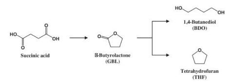
**Figure 5.** Reaction of succinic acid into 1,4-butanediol to produce PBS [46]. Adapted with permission from Delhomme (2009).
