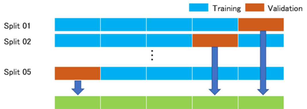
Figure 1 K-Fold ( K = 5 ) cross validation method. All images are divided into five groups. Four groups are augmented and then used for training the model, and one group is used as a validation data. The process repeated five times until each of the five groups becomes a validation data. The answers of the neural networks for all images are used for calculating the performance of the neural networks.
