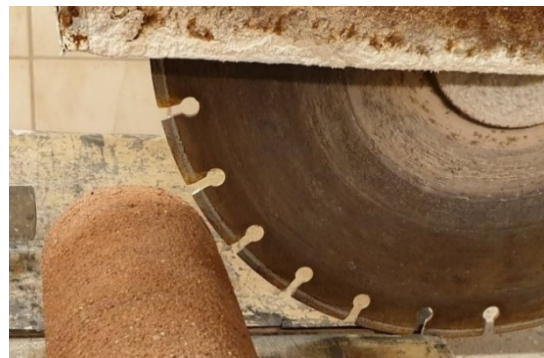
Figure 5. Method of preparing the discs from the cylinder.
