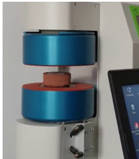
Figure 8. Thermal conductivity test of one of the CSRE samples in FOX 50 plate apparatus.
