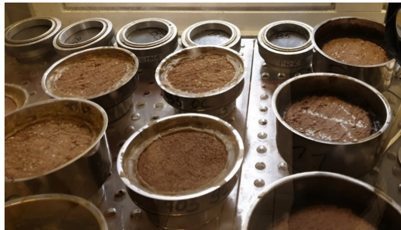
Figure 7. Vapour permeability test.
