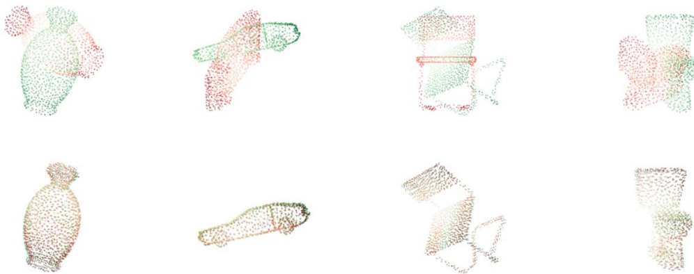
Figure 2. Registration results (red: source point cloud, green: template point cloud). The initial positions of the two point clouds are shown at the top and the results of the alignment are shown at the bottom. It can be seen that the proposed network can also achieve good registration results for methods that may fall into the local optimal solution due to the highly symmetric point cloud.
