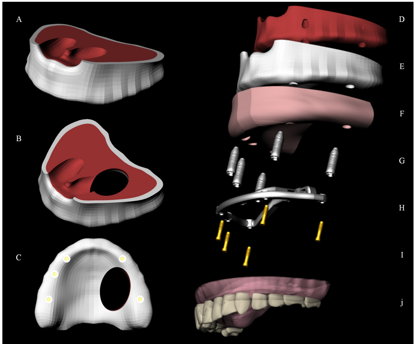
Fig 2. 3D model and geometries. Edentulous maxilla (A); Type IIb maxillary defect (B); Implants distribution on maxillary crestal bone (C); Cancellous bone (D); Cortical bone (E); Soft tissue (F); Five external hexagon implants (G); Bar and bar-clip attachments (H); Five prosthetic screws (I); Full-arch total prosthesis (J).
