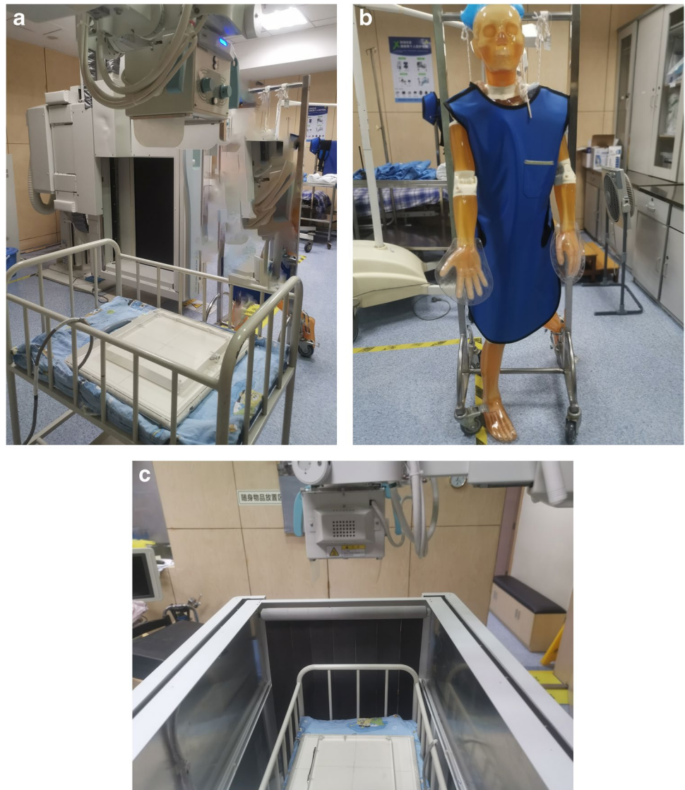
Fig. 2 Clinical images of the three protection scenarios for scatter radiation: (a) no protection, (b) protection with radiation personal protective equipment and (c) the protective trolley for newborns
