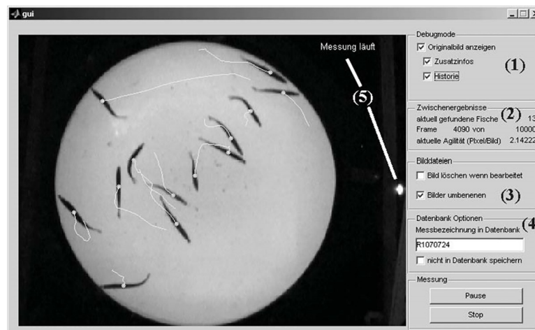
Fig 3. Graphical user interface (GUI). GUI of the fish-tracker for the automated tracking of sprat in an intermittent-flow respirometer. During the processing it was possible to show the original images with the option to display the centre points of each fish and the tracking history of the last twelve images as lines (1). Information on the actual tracked image (2) was given below. Image processing options (3) and database options (4) had to be adjusted before the start of the program. The IR-LED was powered only during measuring phases (5).
