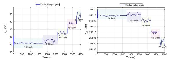
**Figure 18.** Results of fuzzy logic estimator, effective radius,  $R_{eff}$ , and contact length,  $cl_w$ .
