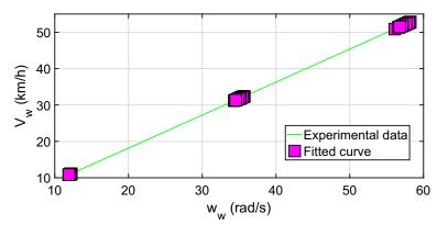
**Figure 14.** Relationship between tire speed,  $V_w$ , and rotation speed,  $\omega_w$ , calculated through the methodology proposed in the experimental data.
