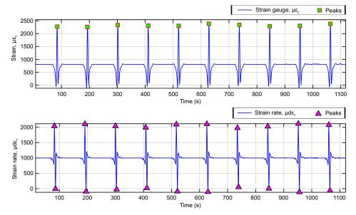
**Figure 5.** Selection of the deformation characteristics in the time history of the deformation in the circumferential direction ( $\varepsilon_x$ ), and its derivative curve ( $d\varepsilon_x$ ) Operating conditions: 0.8 *bar*, 0°, 50 km/h, 500 N.
