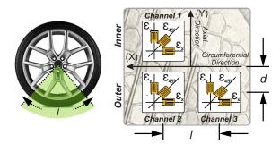
Figure 2. Disposition of the multiaxial gauge strain [28].
