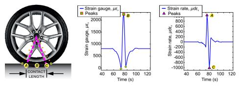
**Figure 6.** Characteristics of the contact trace on the circumferential strain curve ( $\varepsilon_x$ ) and on the derived strain curve ( $d\varepsilon_x$ ). Operating conditions: 0.8 *bar*, 0°, 50 km/h, 500 N.
