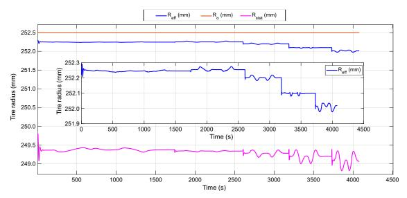
**Figure 19.** Comparison between the estimated effective radius,  $R_{eff}$ , the static radius,  $R_{stat}$ , and the undeformed radius,  $R_o$ , of the tire under the DLC maneuver at different speeds.
