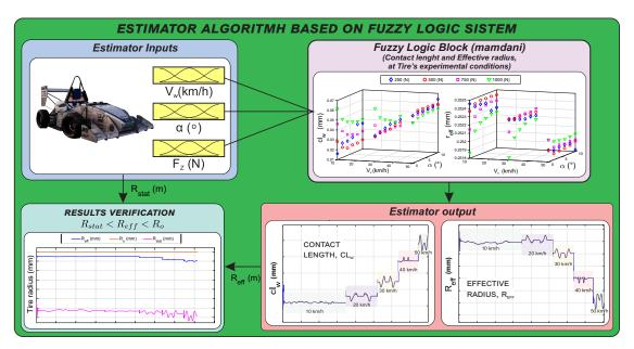
Figure 15. Algorithm of the development of the fuzzy logic estimator.
