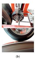
**Figure 1.** Test procedure applied to the intelligent tire: (a) The coordinate system used on the indoor tire test rig; (b) Instrumented tire set up on the tire test rig and its contact with the drum's surface.
