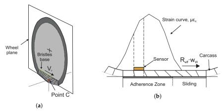
**Figure 9.** Hyphoteses of the strain measurement. (a) Example of the velocity in the base point of the bristle; (b) Ilustrations of the strain measurement for a tire bristles in the adhesion zone.
