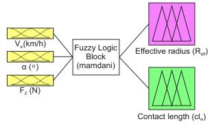
Figure 16. Estimator architecture developed through fuzzy logic.
