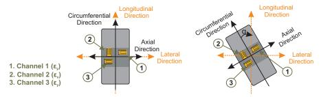
Figure 7. Main measuring direction of the strain sensors.
