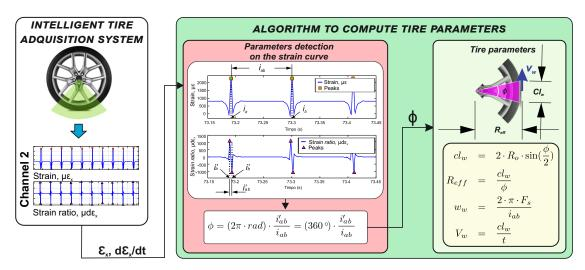
**Figure 4.** Workflow for the development of the intelligent tire detection algorithm.
