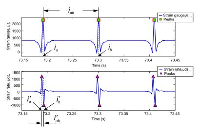
Figure 10. Calculation of the contact length using the strain curve in the circumferential direction (0.8 bar,  $0^{\circ}$ , 50 km/h, 500 N).
