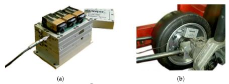
**Figure 3.** Acquisition system SoMat<sup>®</sup> 2000: **(a)** Microprocessor for the data acquisition, and a Power/Communication module; **(b)** Data acquisition module installed on the tire [28].
