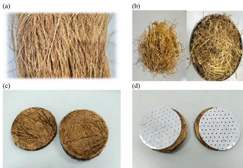
**Fig. 2.** Test SG specimens of (a) dry SC fiber with its average length of 5 cm and weight of 50 g, (b) 50 g of dry SC fiber placed in a metal mold before pressing, (c) pressed SG specimens without covered with PAS and (d) pressed SG specimens covered with PAS.
