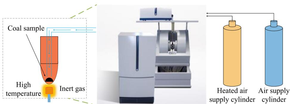
**Figure 4.** Illustration of the blocking pressure testing system.
