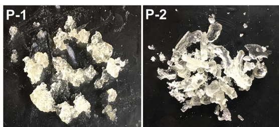
Fig. 4 Silicones prepared following the 1-catalyzed hydrosilylation of vinyl-terminated poly(dimethylsiloxane) (P-1) and 1,2,4-trivinylcyclohexane (P-2) using PMHS.
