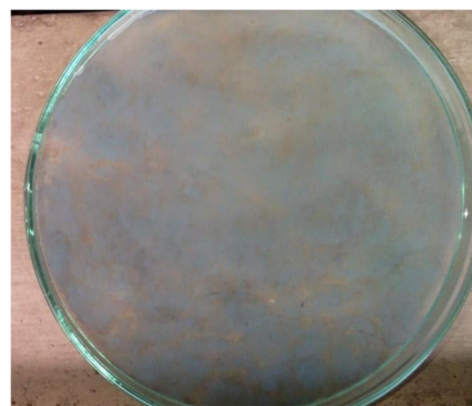
Figure 4. Synthesized nano-ZnO–CuO alginate showing ZnO NP and CuO NP dispersed in Zn–Cu alginate matrix. This hydrogel showed a combination of properties of both nano-ZnO hydrogel and nano-CuO hydrogel.
