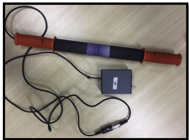
Fig. 2. Roller massage device used. This device was 18 cm in length and 3 cm in diameter with a dense rubberized surface, and it had strain gauges affixed to the roller rod to transmit the signal via Bluetooth to a computer, allowing to control the magnitude of force applied during the intervention.
