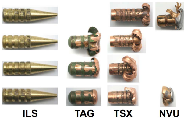
Figure 8. Exiting fragments. The exiting fragments were collected and weighed to calculate the deposited energy. Fragments are shown for increasing speeds from top to bottom. Pictures were only taken when fragments exited the soap block. doi:10.1371/journal.pone.0102015.g008
