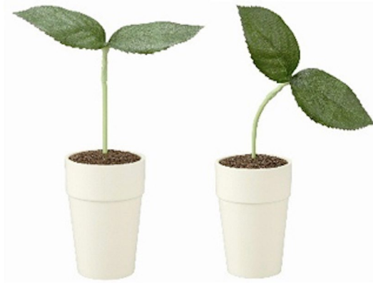
Figure 1. Toy Robot "Pekoppa". The toy robot was used as free of culture or nation affiliation. Pekoppa is the simplest expression of Sakura, which is a voice-driven group of humanoid entrainment systems that reacts to speech sounds by only nodding.
