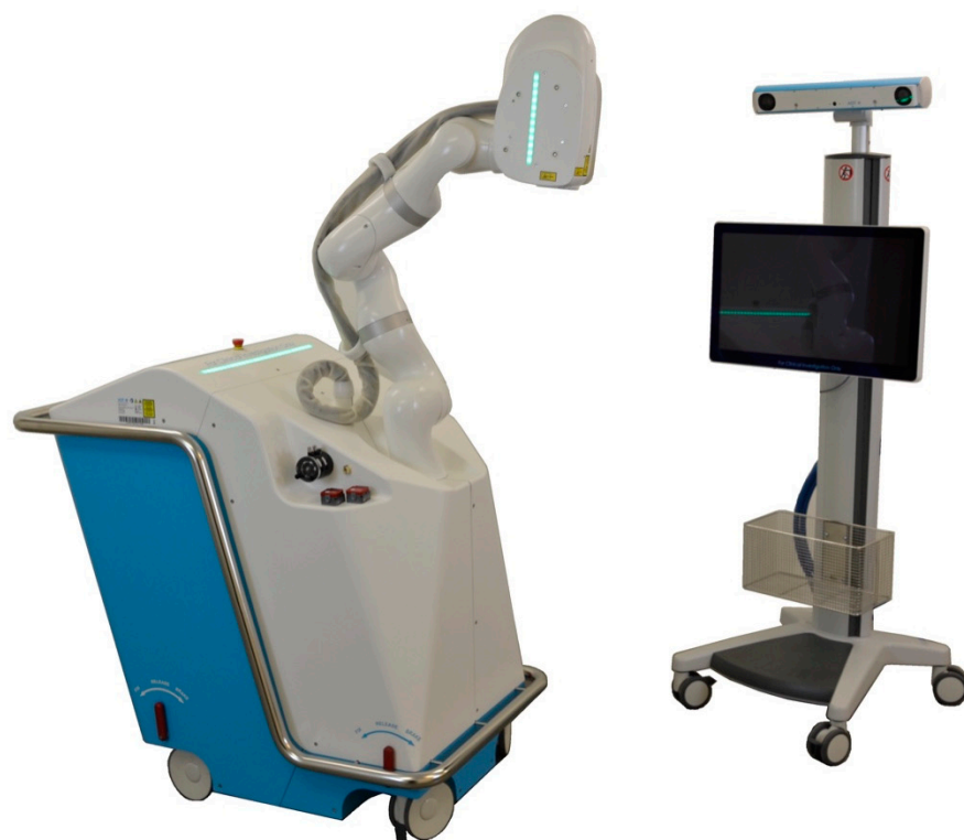
Figure 1. Cold Ablation Robot-guided Laser Osteotome (CARLO ® ) developed by Advanced Osteotomy Tools (AOT AG, Basel, Switzerland) consisting of a laser head mounted on a robotic arm and guided by an optical navigation system.
