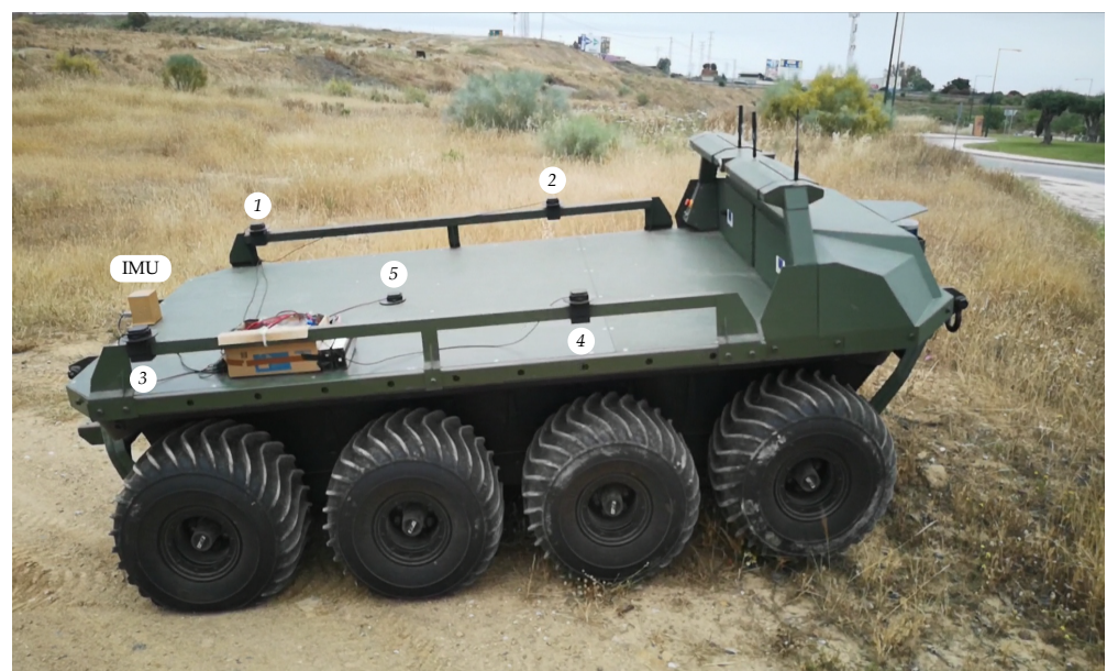
Figure 7. The rover Argo XTR with the sensor system mounted on the rear deck. GNSS antennas are numbered from 1 to 5.
