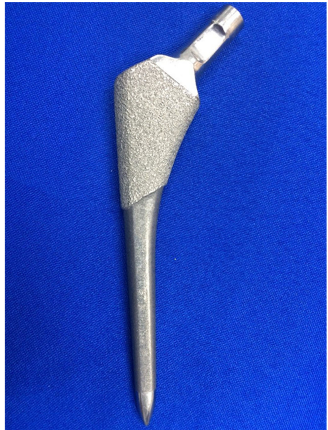
Fig. 1 The stem used in this study: An Echo Bi-Metric RPP stem, which was a collarless 3° bi-planer tapered stem made of titanium alloy. The neck angle of the stem was 135°. The proximal part was porous-coated with a plasma-sprayed high activity (HA) layer, and the distal part was polished and bullet-shaped.
