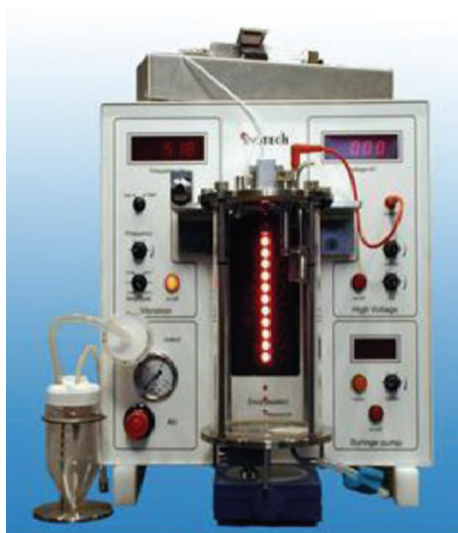
FIGURE 1: Encapsulator for making uniform gel beads.
