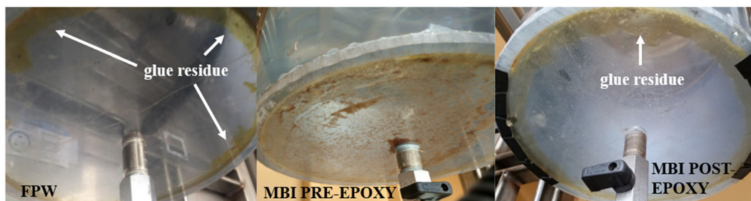
FIGURE 6 Particulates were not observed settled at the bottom of the constant-head reservoir by the end of the column trials at the advanced water purification facility (AWPF) site where the columns were fed with finished product water (FPW). For columns fed with water from the end of the 6-km pipeline at Mid-Basin Injection (MBI pre-epoxy) well site prior to epoxy application, brownish, fine, sand-like particulates were observed settled at bottom of the constant-head reservoir after each trial. After epoxy was applied, subsequent column trials at the MBI site (MBI post-epoxy) did not show fine particle matter settled at the bottom of the constant-head reservoir. The colored ring surrounding the edges of the reservoir is discolored glue residual, not biological growth.
