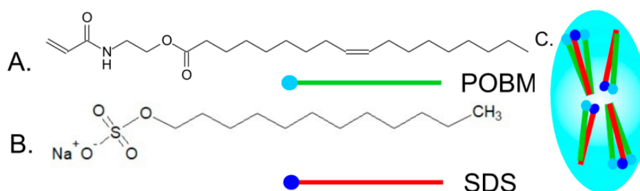
Figure 14. Chemical structure of plant oil-based monomer (A), surfactant (B), and schematic of POBM solubilization by SDS molecules (C). Reprinted from [36]. Copyright (2019), with permission from Elsevier.
