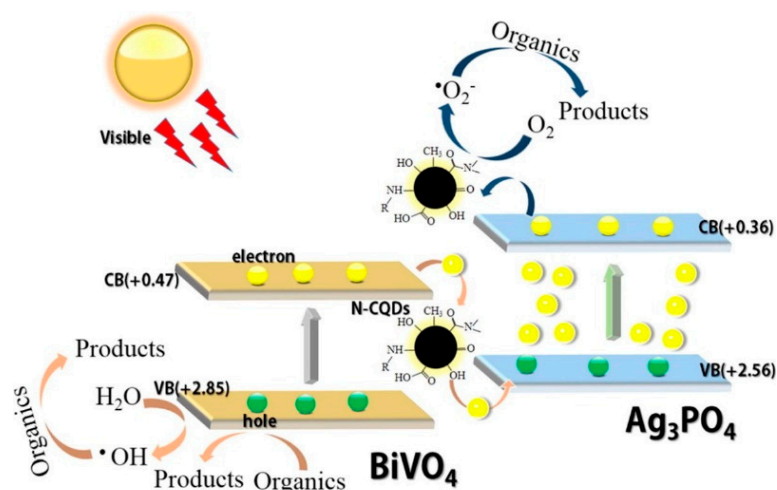
Figure 7. A schematic mechanism of Z-schemed NCDs/Ag 3 PO 4 /BiVO 4 photocatalyst to degrade organics. Figure adapted from reference [117].
