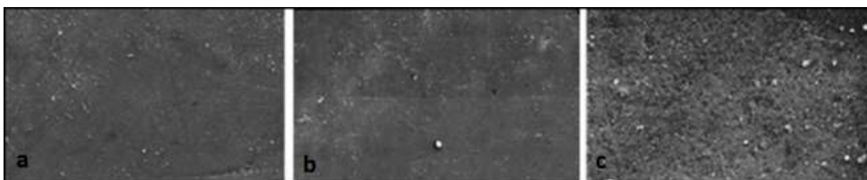
Fig. 4. Scanning electron micrograph of the surface of a Renamel specimen after polishing with Opti1Step system. (a) Original magnification \times 300 . (b) Original magnification \times 700 . (c) Original magnification \times 3000 . In all magnifications, a homogenous and tenacious resinous smear layer can be seen that formed during polishing. At \times 700 magnification, some rubber remnants are seen
