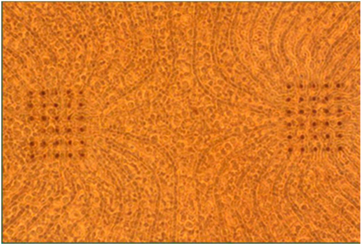
Figure 1. Phase contrast micrograph of the high-density electrode array, on which healthy neurons are growing. The HD array consists of two 6 \times 5 electrode grids ( 10 \mu\text{m} diameter, 30 \mu\text{m} spacing). The distance from center-to-center of the two electrode arrays is 200 \mu\text{m} .
