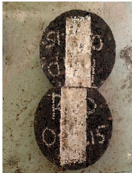
Figure 6. Saw-cut specimens for HWTD.
