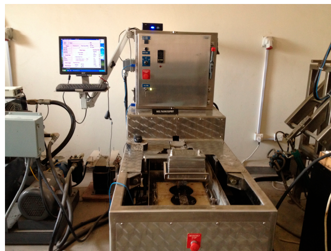
Figure 8. Hamburg Wheel Tracking Device and specimen setup.
