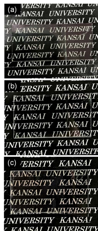
Fig. 2 Optical micrographs of the WO 3 (a), Sn-WO 3 (b), and In-WO 3 (c) films heated at 500 °C.
