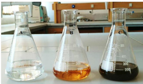
Figure 2. Synthesis of AgNPs by using extract of Carya illinoensis : a) Precursor solution of AgNO 3 , b) Extract of Carya illinoensis , and c) Extract of Carya illinoensis treated with AgNO 3 .
