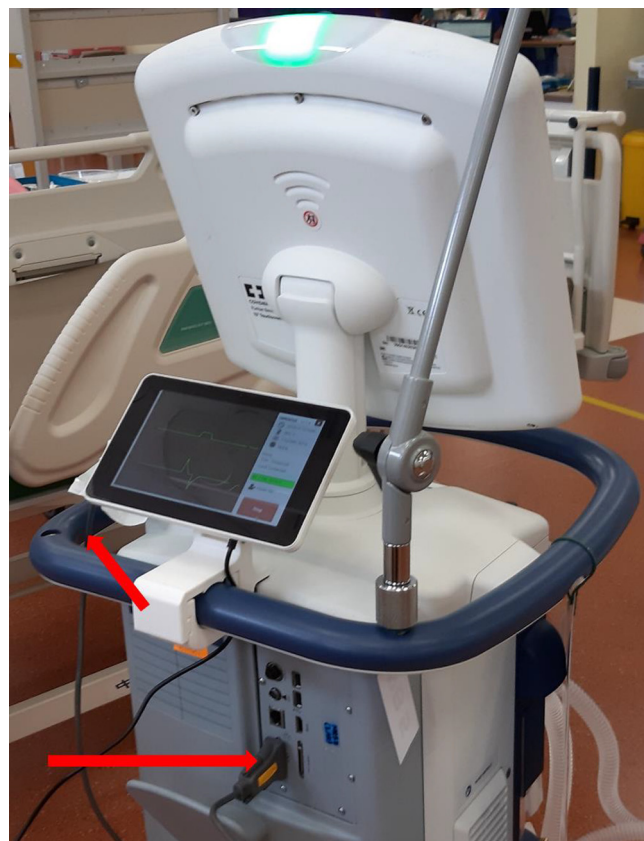
Fig. 8. Figure of DAQ assembly mounted on the railing of the ventilator. The USB to Serial cable is connected to the Raspberry Pi and ventilator, respectively (Red arrows). (For interpretation of the references to colour in this figure legend, the reader is referred to the web version of this article.)
