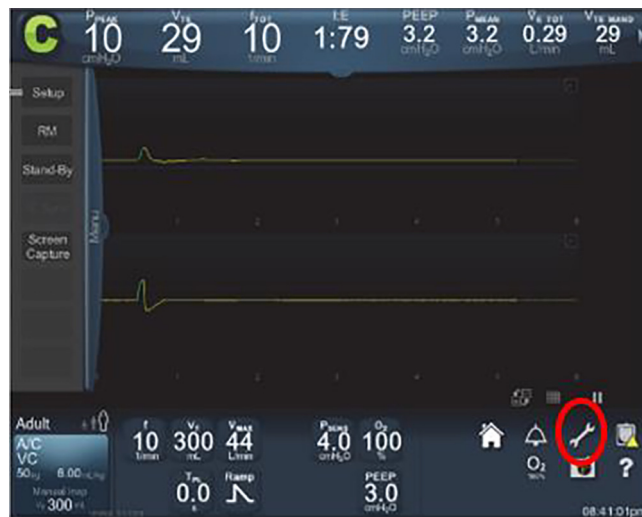
Fig. 9. Main ventilator screen of the ventilator interface. Settings page is accessed via clicking on the Settings button (Red Circle). (For interpretation of the references to colour in this figure legend, the reader is referred to the web version of this article.)
