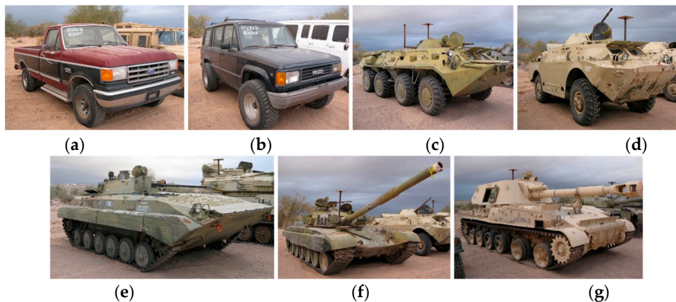
Figure 4. Seven targets in SENSIAC: (a) Truck; (b) SUV; (c) BTR70; (d) BRDM2; (e) BMP2; (f) T72; and (g) ZSU23-4.
