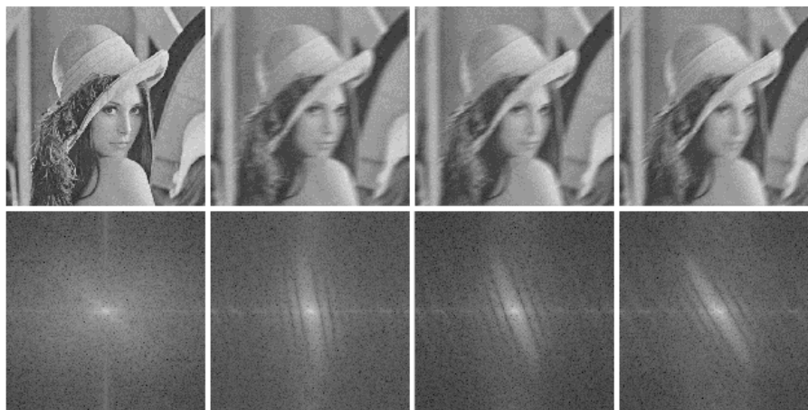
Figure 1. Figures from left to right are: original image with no motion, 20°, 40°, 60° movement in the horizontal direction. The figures below are their corresponding spectrum.
