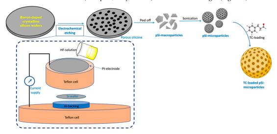
Figure 1. Schematic illustrating the synthesis of the pSi-TC microparticles.
